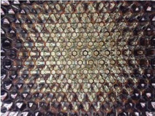
Part of the photosensor array, with light collecting funnels in front of the photomultiplier tubes (Credit: H.E.S.S. Collaboration, Arnim Balzer)
