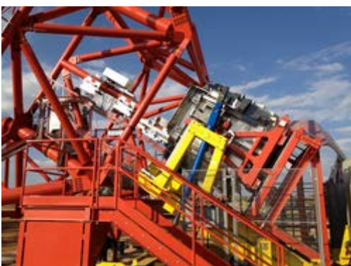
The "camera" with photosensors and readout electronics is loaded into the nose of the telescope (Credit: H.E.S.S. Collaboration, Arnim Balzer)
